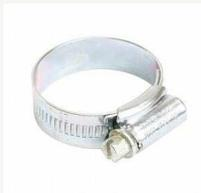
When connecting flexible duct to solid components jubilee/speed clamps should be used to ensure tight fixings which are free from movement. This is also recommended when attaching duct to exhaust and extract terminations.
